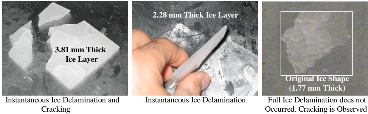
Figure 11: Experimental Ice De-Bonding and Fracture Patterns under Ultrasonic ZX and XY Shear Stresses (28.5 KHZ, 50 V, -20° C). Patterns Agree with FEM Predictions
